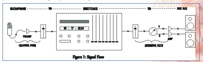
How can a recorder play back one thing while recording another? Simple enough. Each track of the multitrack recorder assumes one of two states: playback or record. When a track is in the playback mode, its audio is sent to the multitrack machine's output. In record mode, new audio for that track is written/stored on the tape or disk.
