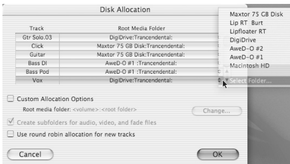
Fig. 3.4. The Disk Allocation window enables you to choose the exact location where each track you record will be stored. To assign all tracks to a specific drive, press Alt (Win) or Option (Mac) while selecting a drive name.
